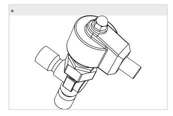
When a sudden change in the thermal load occurs, a traditional expansion valve is designed to be in a transient state for 2-3 minutes before reaching its equilibrium condition. E.g.:
