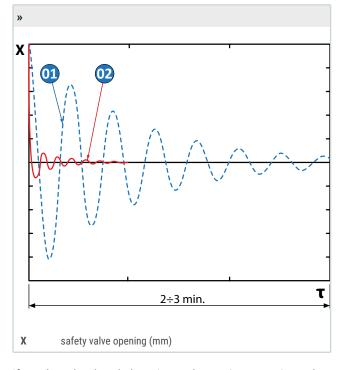
If, on the other hand, there is an electronic expansion valve, in case of a compressor switch on or off request:
