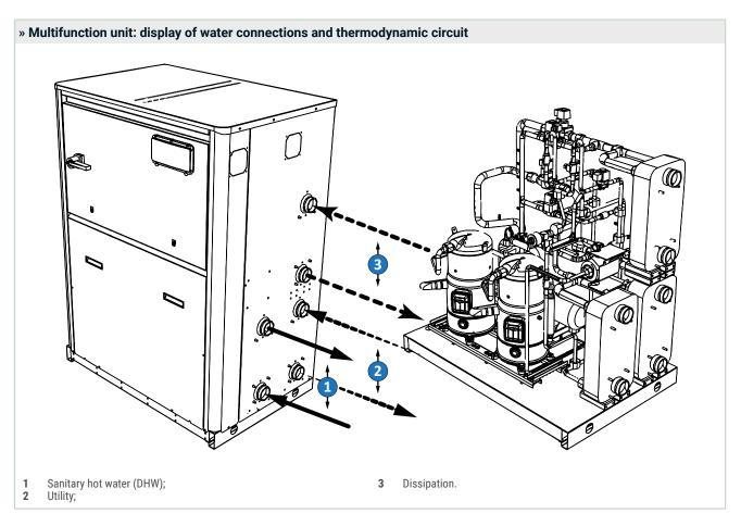
ENP units make it possible to install indifferently a simple 2 or 4 pipe air conditioning system. The two or four pipe designation refers to a water distribution system supplying each air conditioning appliance of a building. A 2-pipe system (ENP M) includes one supply line and one return line to the unit. The terminals supplied by a 2-pipe system have
