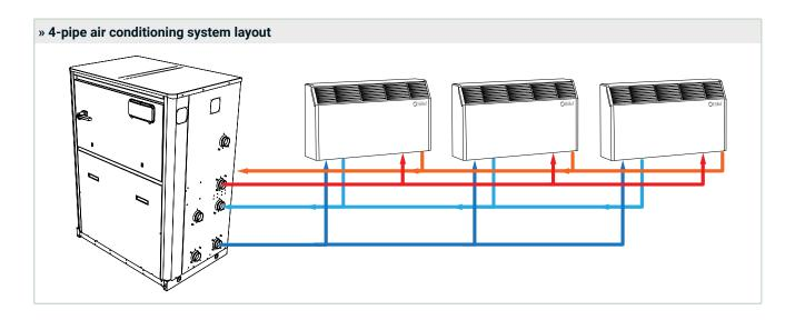
The 2-pipe systems are less flexible than 4-pipe systems because the entire building is either heated or cooled, though the installation greatly saves energy.
