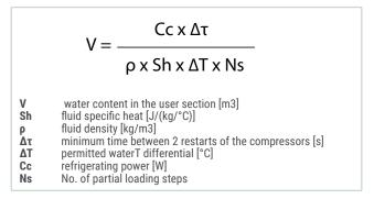
The following figure shows the integrated and balanced effect of the storage tank. Its function helps ensure accurate temperature control according to the environmental parameters of the connected groups.
