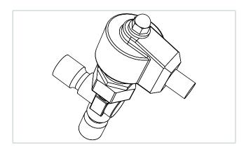
When a sudden change in the thermal load occurs, a traditional expansion valve is designed to be in a transient state for 2-3 minutes before reaching its equilibrium condition. E.g.:
