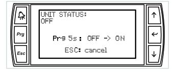
Press the key **PRG** for 5 seconds to switch the status of the machine or press the key **ESC** to exit without changing the status.
