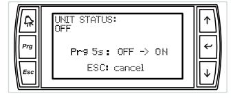
Press the key **PRG** for 5 seconds to switch the status of the machine or press the key **ESC** to exit without changing the status.
