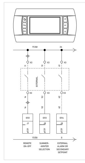
The user interface, PCO, consists of an LCD display and 6 keys. All the program operations can be run, the conditions of the operating unit can be displayed at any time and the parameters can be modified.
